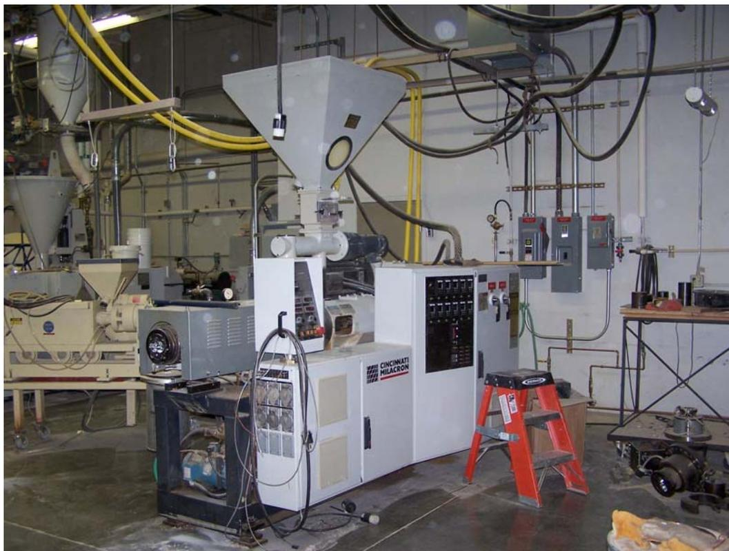
Figure 4.8 : Extrudeuse Cincinnati Milacron du Laboratoire de Washington State University.
